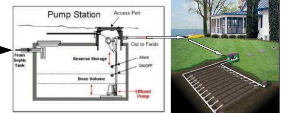
From the Pump Tank it's transferred into the drip irrigation field.
